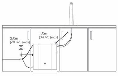
Identify a suitable location for the ProCore unit. It should be positioned within 1.0m of the faucet, and within 2.0m of suitable services connections. Ensure to allow enough space for the Simple-fit Vent Kit which must be installed with the unit.
