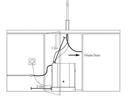
Identify a suitable location for the ProCore unit. It should be positioned within 1.0m of the faucet, and within 2.0m of suitable services connections. Allow enough space to fit the ventilation ducting system.
