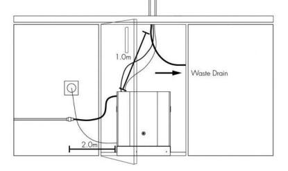
Identify a suitable location for the ProCore unit. It should be positioned within 1.0m of the faucet, and within 2.0m of suitable services connections. Allow enough space to fit the ventilation ducting system.
