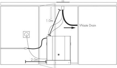
Identify a suitable location for the ProCore unit. It should be positioned within 1.0m of the faucet, and within 2.0m of suitable services connections. Allow enough space to fit the ventilation ducting system.
