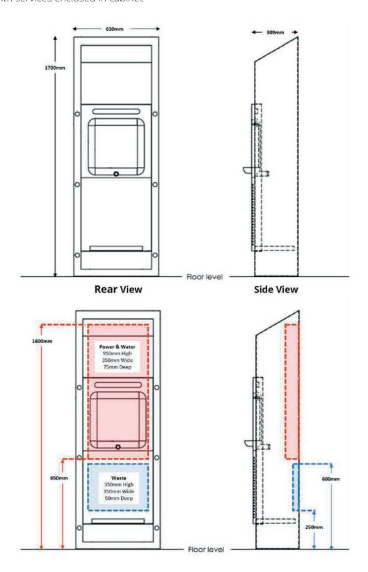
**Important Note:** The waste pipe must not exceed 50mm from the wall where a chiller is fitted
