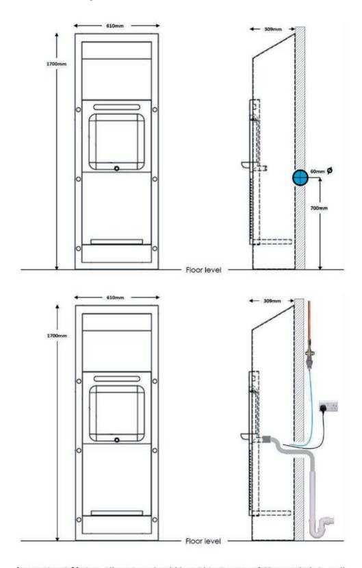
**Important Note:** All services should be within 1 metre of 60mm Ø hole in wall
