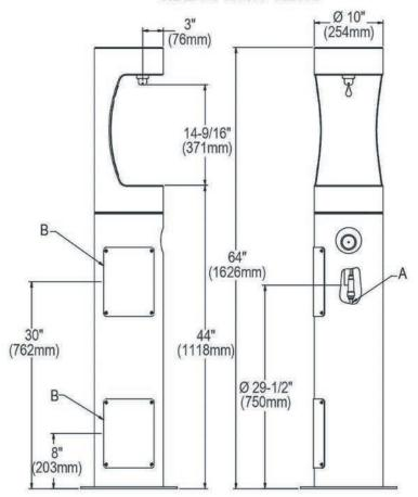
A = 3/8" O.D. Unplated copper tube connect. Shut off valve by others. B = Access panel(8" x 10")
