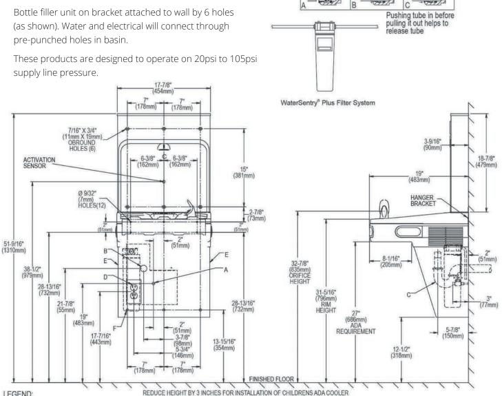
LEGEND: A = Recommended Water Supply location. Shut-off Valve (not furnished) to accept 3/8" O.D. unplated copper tube. Up to 3" (76mm) maximum out from wall. B = Recommended Waste Outlet location. To accommodate 1-1/4" nominal drain. C = 1-1/4" Trap (not furnished).
