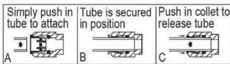
Pushing tube in before pulling it out helps to release tube
