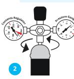
Screw the gas regulator in an anticlockwise motion onto the thread of the canister. As it tightens you might hear a short hiss of gas as the seal is made.
